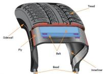
Figure 1: Basic structure of a passenger car tyre. Belts provide stiffness to the tread, overall tyre strength, and protection from puncture; body ply maintains tyre shape and prevents it from tearing; beads enable the tyre to firmly grip to the wheel.
