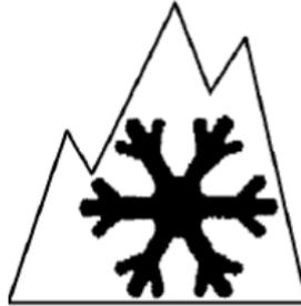
**Sidewall symbol of tyres for use in severe snow conditions.**
