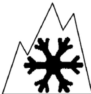
Minimum 15 mm base and 15 mm height, placed adjacent to the M+S type designation. Above drawing not to scale.
